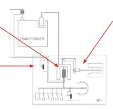
AKM Compensation bellow automatically compensates for ambient temperature
